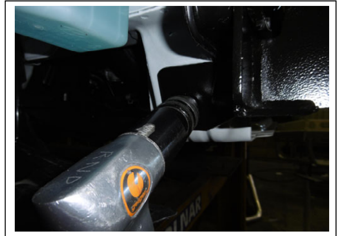
Figure 6: Drill hole in radiator support using steel mounting bracket as a guide.
