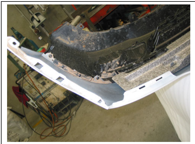
Figure 1: Clips on top edge of bumper to guard and headlight
