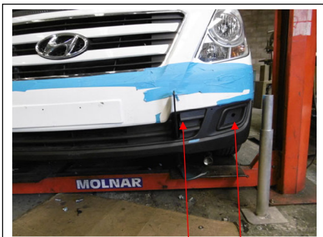
Figure 3: Grille cut out 17mm cutout in blank
