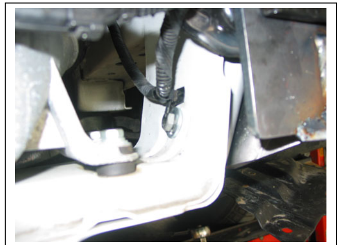
Figure 6: Drill hole in radiator support using steel mounting bracket as a guide.
