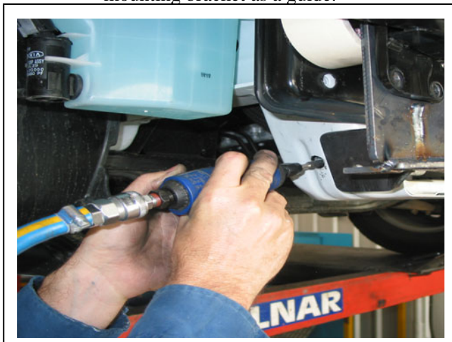
Figure 7: Enlarge hole in radiator support using a die grinder.
