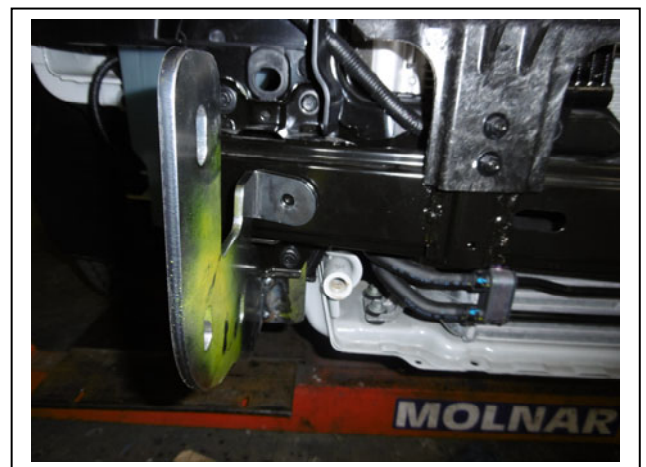
Figure 4: Steel mounting bracket being placed behind bumper support. Drivers's side shown.
